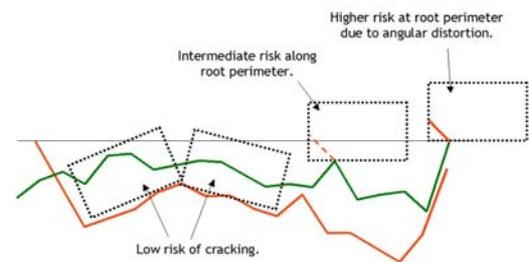
By modelling the relationship between measured ground movement and buildings (see above) it would appear that the fulcrum most likely to result in excessive tensile stresses lies at the periphery of the movement zone.
